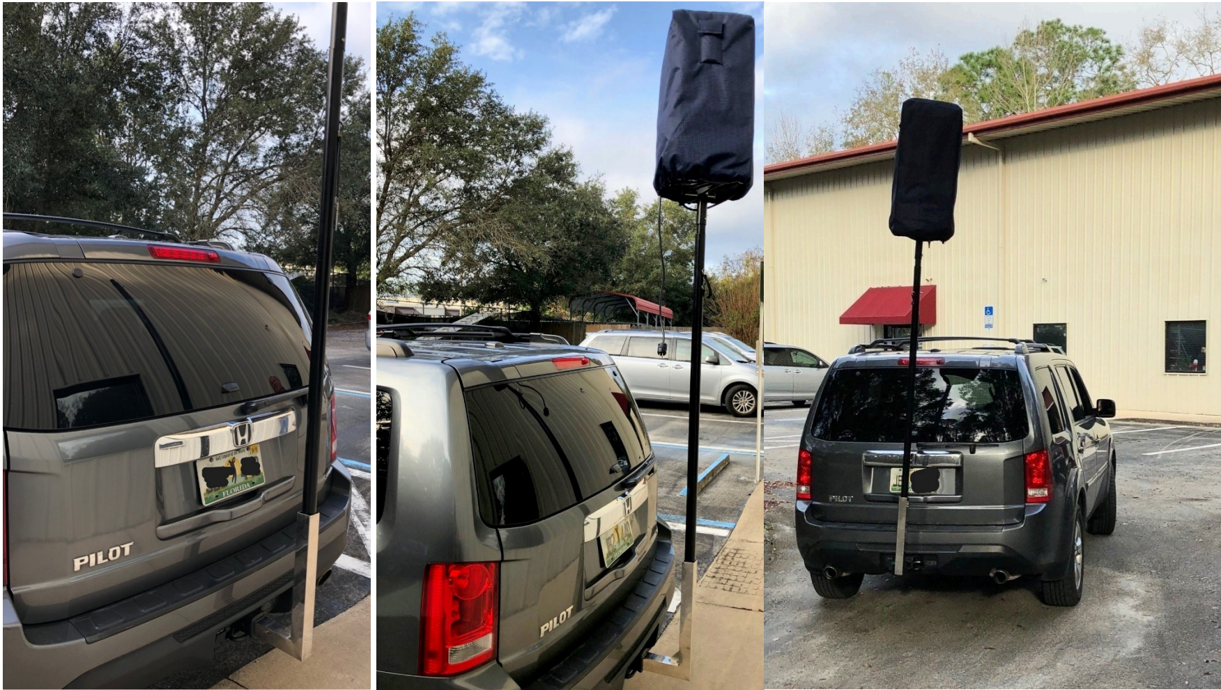
Prism Balloon Light (PBL 500 LED) mounted on a custom hitch
